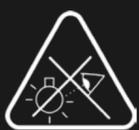
**Caution! Risk group 2:** Possibly hazardous optical radiation! Do not look into the lamp for extended periods during operation, as this can damage the eyes.
